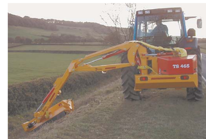
Heavy Duty Reversible Lump Flail for hedging and occasional mowing. This flail is fitted as standard unless otherwise specified.
