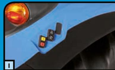
External PTO and hitch controls are located on the rear fenders, making it easier to attach implements from the ground (fig. I).
